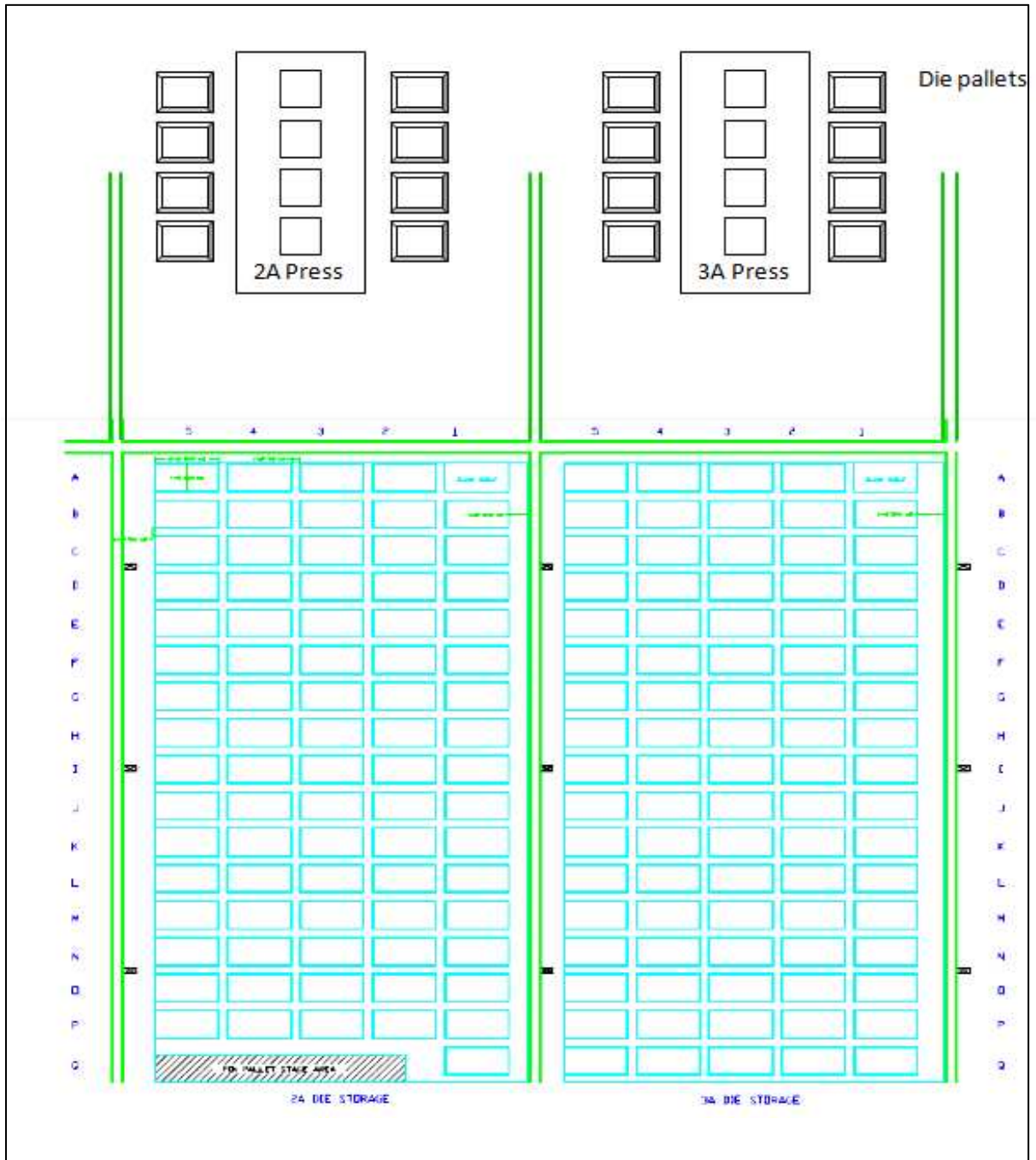
Figure 3 Design layout of Die based storage automotive stamping shop
